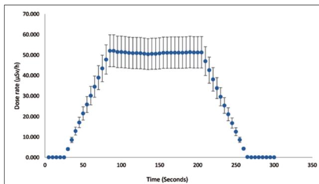
**Fig. 7.** The measured dose rate of the Hopewell  $^{137}\text{Cs}$  source<sup>9)</sup> when it was set at 50  $\mu\text{Sv/h}$ .
