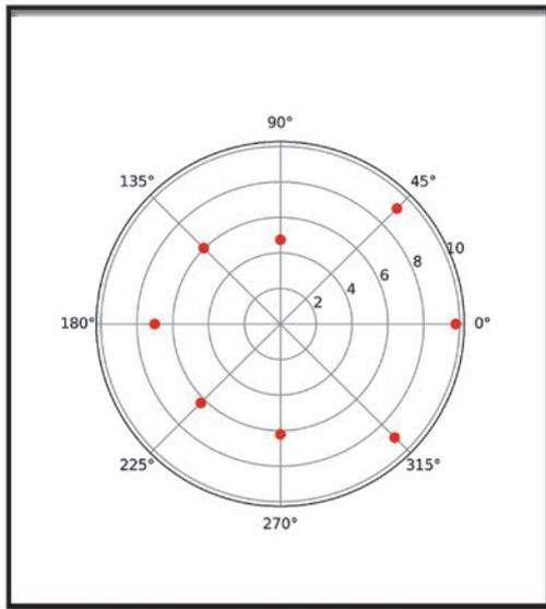
**Fig. 8.** Angular response of the bGeigie Nano Monitor.
