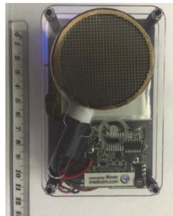
**Fig. 3.** The back of the bGeigie Nano Monitor with the case off. Also note the LND7317 Pancake GM on the back of the monitor.
