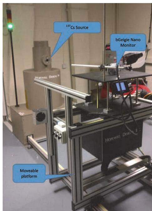
**Fig. 4.** The EPA’s calibration facility<sup>3)</sup>. The bGeigie Nano Monitor can be seen attached to the moveable platform which is in the line of sight of the  $^{137}\text{Cs}$  source<sup>9)</sup>
