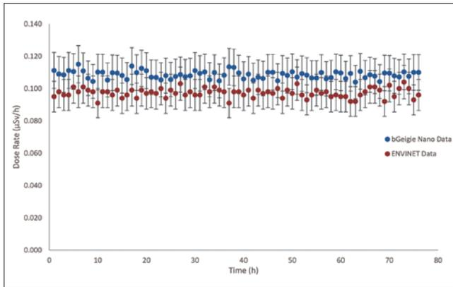
**Fig. 6.** Comparison dose rate measurements between the bGeigie Nano Monitor and the fixed gamma dose rate monitor<sup>(4)</sup> (ENVINET).
