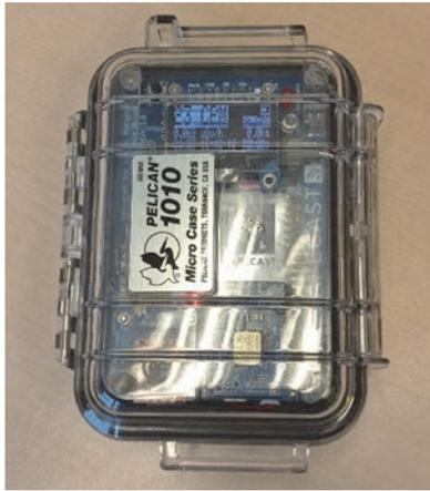
**Fig. 1.** The bGeigie Nano Monitor fully assembled with the case on.
